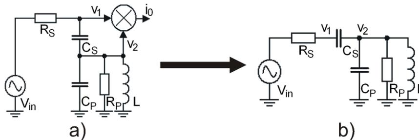
**Fig. 2** a) principle circuit of the quadrature detector, b) quadrature detector model
