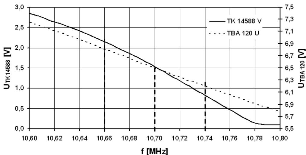
**Fig. 5** Measured S-curves for bit rate 76,8 kbps
