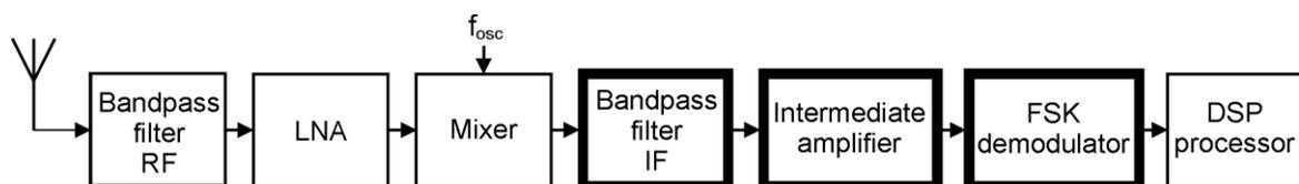
**Fig. 1** Superheterodyne receiver block scheme
