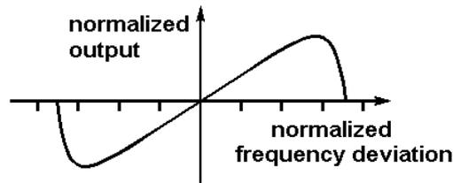
**Fig. 3** S-curve of the quadrature detector
